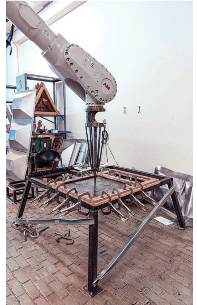
16 Diagram of Robotic Incremental Metal Forming (RIMF) section [Refer to Fig. 17]
